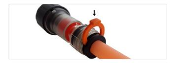
If the Gas Block Connector is not pre-fitted with the locking clip or it has been removed, please insert the correct locking clip of the correct dimension after connecting the Microduct. The insertion of the locking clip between the Gas Block Connector main body and the collet avoids any possibile Microduct accidental disconnection.
