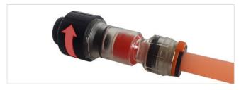
Before the optical fibre cable installation, the Gas Block Connector nut must be completely unscrewed (Open Position). In that position the system is not sealed and the cable can pass through the Gas Block Connector freely.
