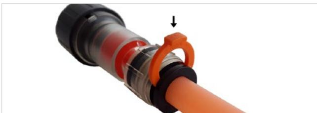
If the Gas Block Connector is not pre-fitted with the locking clip or it has been removed, please insert the correct locking clip of the correct dimension after connecting the Microduct. The insertion of the locking clip between the Gas Block Connector main body and the collet avoids any possible Microduct accidental disconnection.
