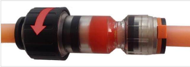
After the cable installation, in order to seal the system and to obtain Gas and Water Block, the nut must be screwed firmly (Closed Position). Do not pull the cable when the Gas Block Connector is in the closed position to prevent possible damage to the gas seal.
