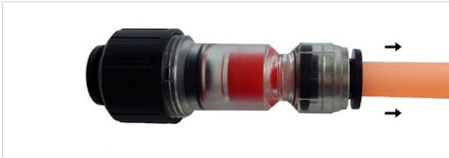
To make sure that the Microduct is properly connected to the Gas Block Connector, please pull it once slightly, without releasing the collet.
