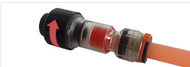
Before the optical fibre cable installation, the Gas Block Connector nut must be completely unscrewed (Open Position). In that position the system is not sealed and the cable can pass through the Gas Block Connector freely.
