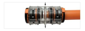
Make sure that the Microduct is correctly and fully inserted. The transparent body of the Connector allows a visual inspection of the correct and full insertion of the Microduct. The insertion of the Microduct into the Connector requires a moderate force. The Microduct and the Connector seal should not be scratched or damaged during the insertion, otherwise there may be leaks or further mis-functioning. Please, connect the Microduct by hand, without using any kind of tool.
