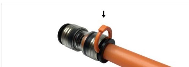
If the Connector is not pre-fitted with the locking clip or if it has been removed, please insert the proper locking clip of the correct dimension after connecting the Microduct. The insertion of the locking clip between the Connector main body and the collet avoids any possible Microduct accidental disconnection.
