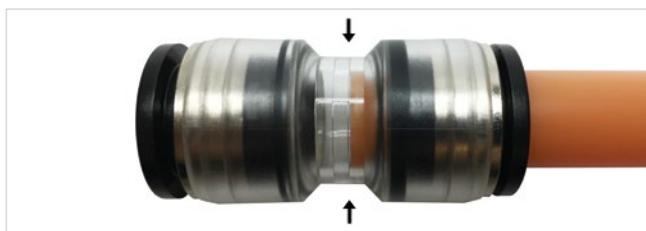
Make sure that the Microduct is correctly and fully inserted. The transparent body of the Connector allows a visual inspection of the correct and full insertion of the Microduct. The insertion of the Microduct into the Connector requires a moderate force. The Microduct and the Connector seal should not be scratched or damaged during the insertion, otherwise there may be leaks or further mis-functioning. Please connect the Microduct by hand, without using any kind of tool.
