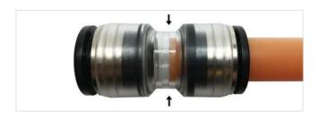
Make sure that the Microduct is correctly and fully inserted. The transparent body of the Connector allows a visual inspection of the correct and full insertion of the Microduct. Insertion of the Microduct into the Connector requires a moderate force. The Microduct and the Connector seal should not be scratched or damaged during the insertion, otherwise there may be leaks or further mis-functioning. Please connect the Microduct by hand, without using any kind of tool.
