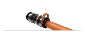
If the Connector is not pre-fitted with the locking clip or if it has been removed, please insert the proper locking clip of the correct dimension after connecting the Microduct. The insertion of the locking clip between the Connector main body and the collet avoids any possible Mircroduct accidental disconnection.
